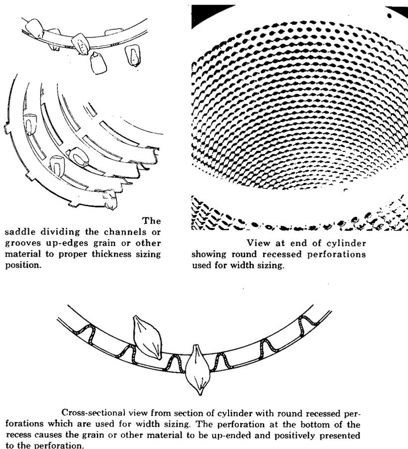
FIGURE 3.—Slotted and round perforations in grader shells.
