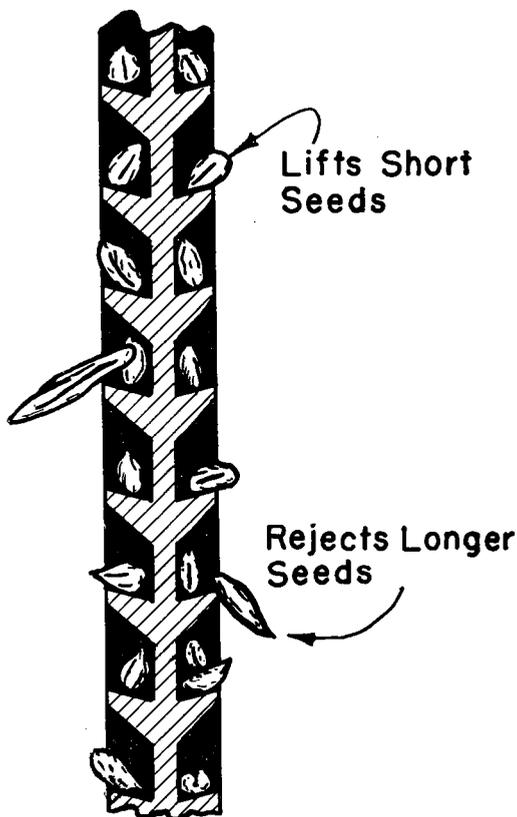
FIGURE 7.—Cross section of an indent disk separator.
