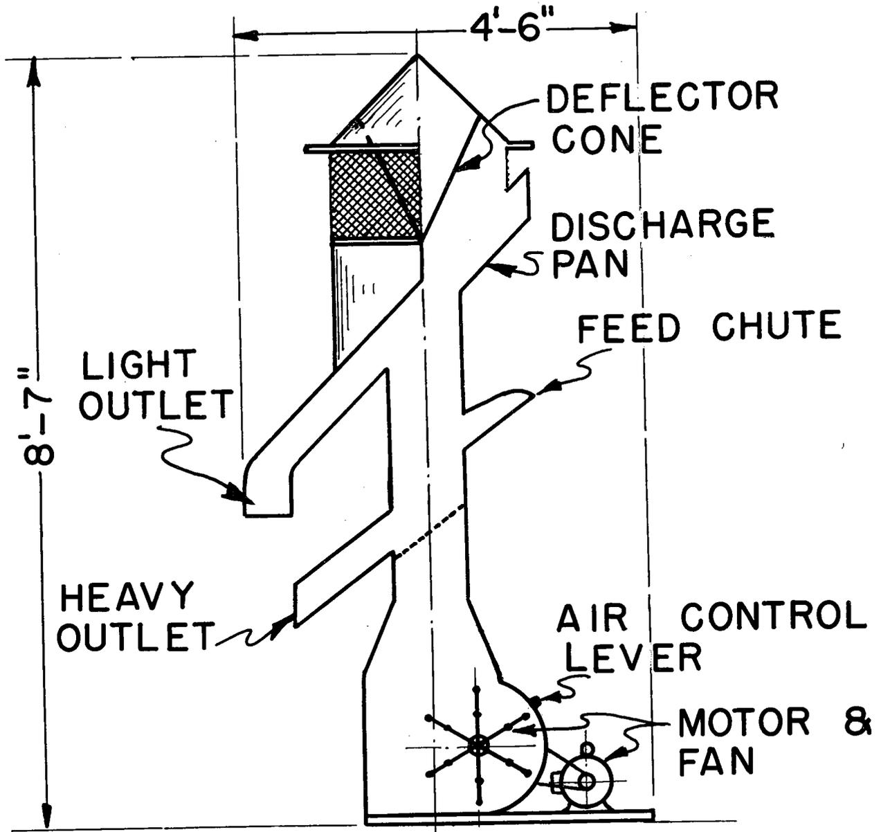
FIGURE 15.—Cross section of pneumatic separator.
