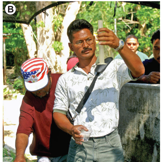
Figure 11.16 —Periodic checks of water distribution can easily be done with a “cup test” in which cups are arranged in a grid pattern (A). The depth of water in the cups is measured after a standard watering period (B). Photo A by Kim M. Wilkinson, and photo B by Thomas D. Landis.
