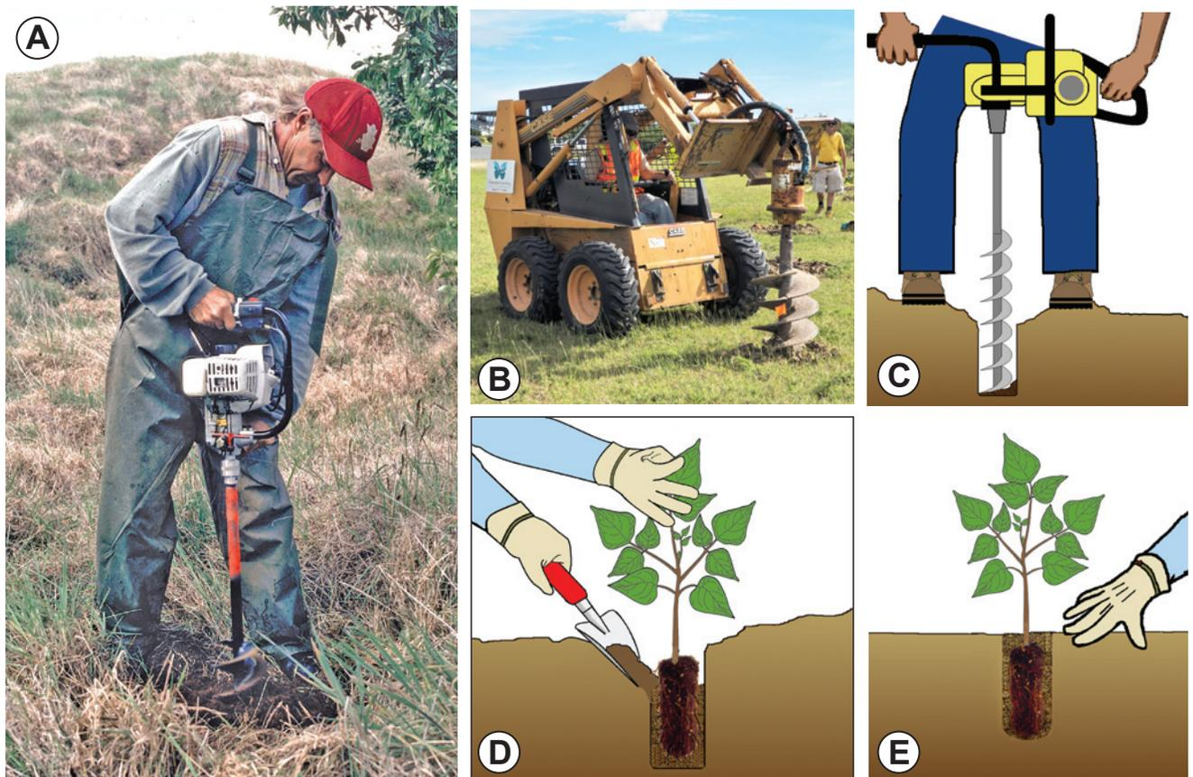
**Figure 17.18**—Augers are effective planting tools and are available in handheld (A) or tractor-mounted (B). One skilled operator can create planting holes (C) while other workers plant the stock and fill the holes by hand (D and E). Photo A by ©Jack Jeffrey Photography, photo B by Brian F. Daley, and illustrations C, D, and E by Steve Morrison, modified by Jim Marin.
