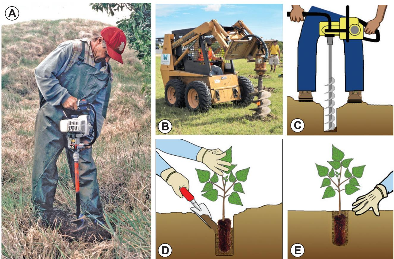
**Figure 17.18**—Augers are effective planting tools and are available in handheld (A) or tractor-mounted (B). One skilled operator can create planting holes (C) while other workers plant the stock and fill the holes by hand (D and E). Photo A by ©Jack Jeffrey Photography, photo B by Brian F. Daley, and illustrations C, D, and E by Steve Morrison, modified by Jim Marin.
