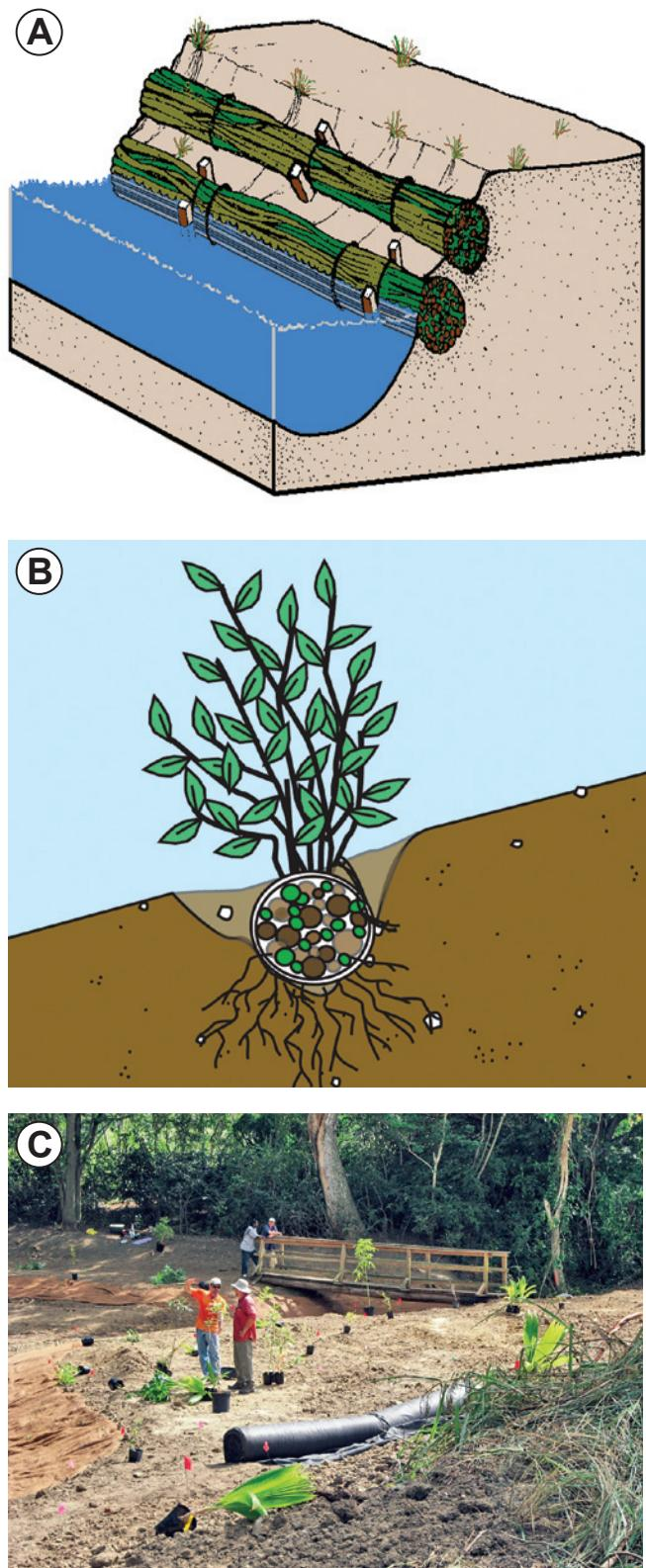
**Figure 17.7**—Stream banks often require bioengineering structures (A) for stabilization. When cuttings of certain species are used, they can sprout quickly (B). Careful planning and quality planting stock help ensure restoration success (C). Illustration A from Hoag and Landis (2001), illustration B from Steinfeld and others (2008), and photo C by Brian F. Daley.
