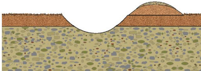
**Figure 17.5**—On sites with heavy duff layers or in waterlogged soils, mounding has proven to benefit plant survival and growth. Illustration from Landis and others (2010).
