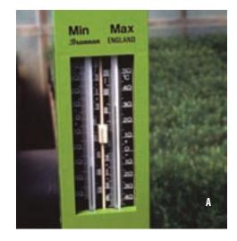
**Figure 4.17**—(*A*) Monitoring and controlling temperature is critical to successfully growing a crop of native plants, and monitoring equipment is inexpensive. Many nurseries use thermometers that record daily maximum and minimum temperatures and (*B* and *C*) small, programmable, self-contained temperature sensors. Photo A by Thomas D.Landis, B and C by David Steinfeld.
