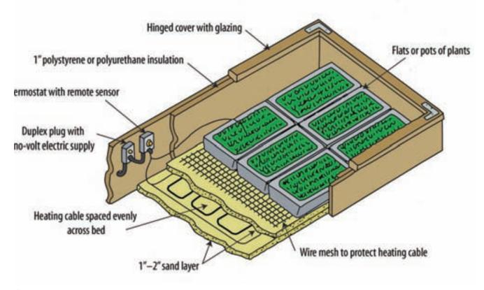
Figure 4.6—A hot bed is structurally similar to a cold frame but is heated by electric heating cables. Illustration courtesy of John W. Bartok, Jr.
