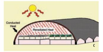
**Figure 4.13**—(*A*) Sunlight provides the energy necessary for plant growth but is converted to heat inside propagation structures. (*B*) By reducing light intensity, shadecloth cools the environment. (*C*) Black shadecloth absorbs heat that is radiated back into the propagation environment, but (*D*) new aluminized shadecloth diffuses light without generating heat. Photos by Thomas D. Landis, illustrations by Jim Marin.
