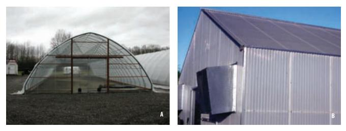
**Figure 4.10**—(*A*) Greenhouses are covered with transparent coverings such as plastic sheeting or (*B*) hard plastic panels to maximize the amount of sunlight reaching the crop. Photo A by Tara Luna, B by Thomas D. Landis.
