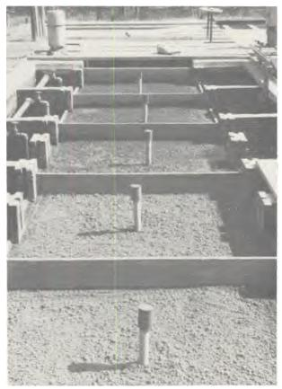
FIGURE 1. An end view of five of the growing comportments of the hydro-edaphytron just prior to planting seedlings in 1965. Flood tanks abut each compartment on the left and right side.
