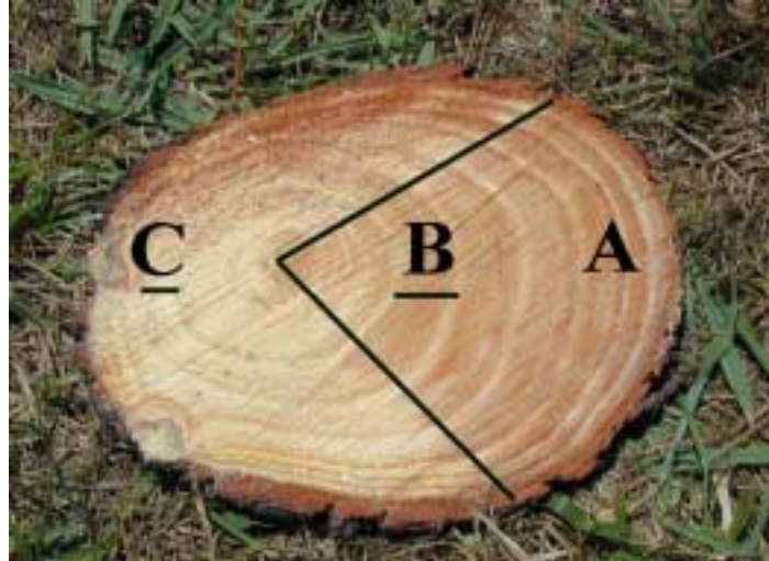
Figure 1. Cross-section through a zone of compression wood in loblolly pine. What was the underside of the stem is clearly demarcated by the darker (reddish) colored wood (A). The eccentric nature of the annual growth rings is highlighted by the bars depicted beneath the lettering (B) and (C).
