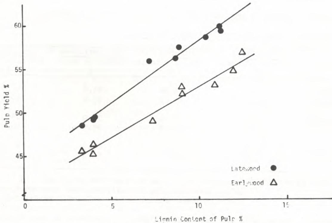
Figure 2. Regressions of Tree 2 (loblolly pine) earlywood and latewood pulp yields on lignin contents of the respective pulps. Yields are expressed on an oven-dry, extracted wood basis. From Gladstone, et al. (1).
