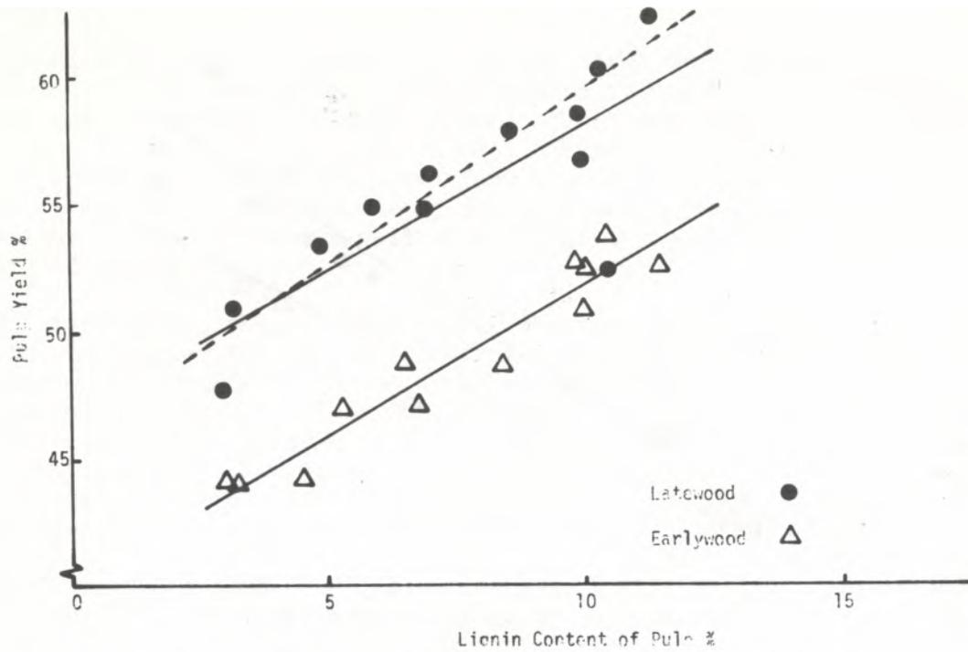
Figure 1. Regressions of Tree 1 (loblolly pine) earlywood and latewood pulp yields on lignin contents of the respective pulps. Dashed line represents latewood regression calculated after excluding outlying point at 10.5 percent lignin content. Yields are expressed on an oven-dry, extracted wood basis. From Gladstone, et al. (1).
