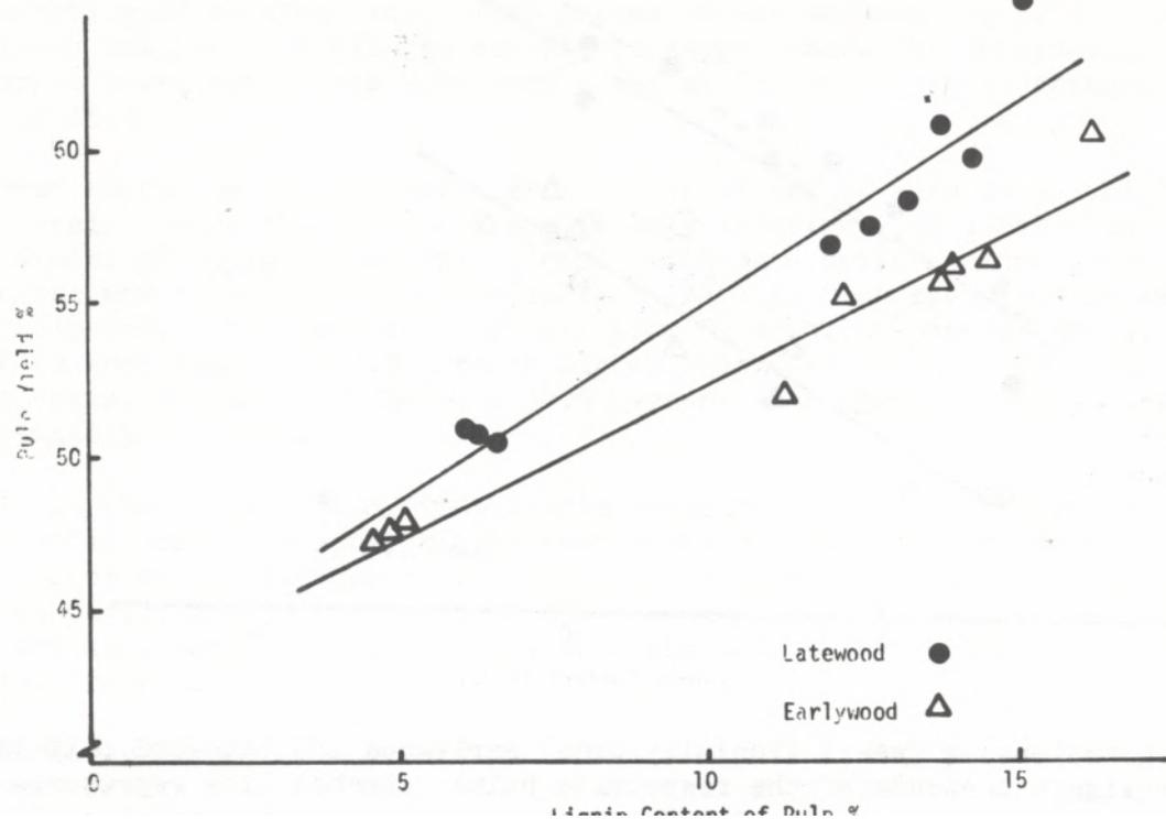
Figure 3. Regressions of Tree 3 (loblolly pine) earlywood and latewood pulp yields on lignin contents of the respective pulps. Yields are expressed on an oven-dry, extracted wood basis. From Gladstone, et al. (1).
