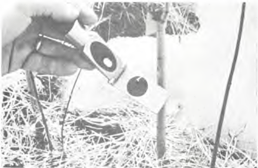
Figure 2. -- To determine the sugar content, a drop of sap at the end of a hypodermic needle is collected on a refractometer plate.
