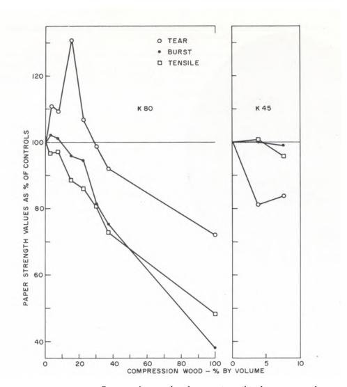
FIGURE 6. — Compression wood and paper strength values expressed as a percentage of the control values.
