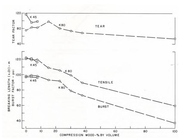
FIGURE 5. — Compression wood content and paper strength.
