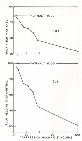
FIGURE 7. — (a) Compression wood content and screened pulp yield; (b) compression wood content and screened pulp yield expressed as a percentage of the yield from "normal" wood.
