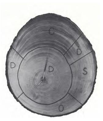
FIGURE 4. — Delineation of discs for pulp and paper-making tests. C is taken to be 100-percent compression wood. S (sidewood) and 0 (opposite wood) are taken as no compression wood; these were combined to give "normal" or control fraction. D is discarded as containing varying amounts of compression wood.
