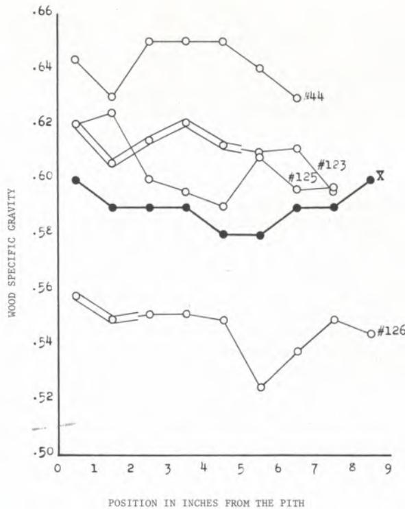
FIGURE 8. — Variation in specific gravity at breast height in relation to position for the average of all trees and for four selected individual trees. The double lines indicate the amount of heartwood.
