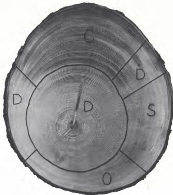
FIGURE 4. — Delineation of discs for pulp and papermaking tests. C is taken to be 100-percent compression wood. S (sidewood) and O (opposite wood) are taken as no compression wood; these were combined to give "normal" or control fraction. D is discarded as containing varying amounts of compression wood.
