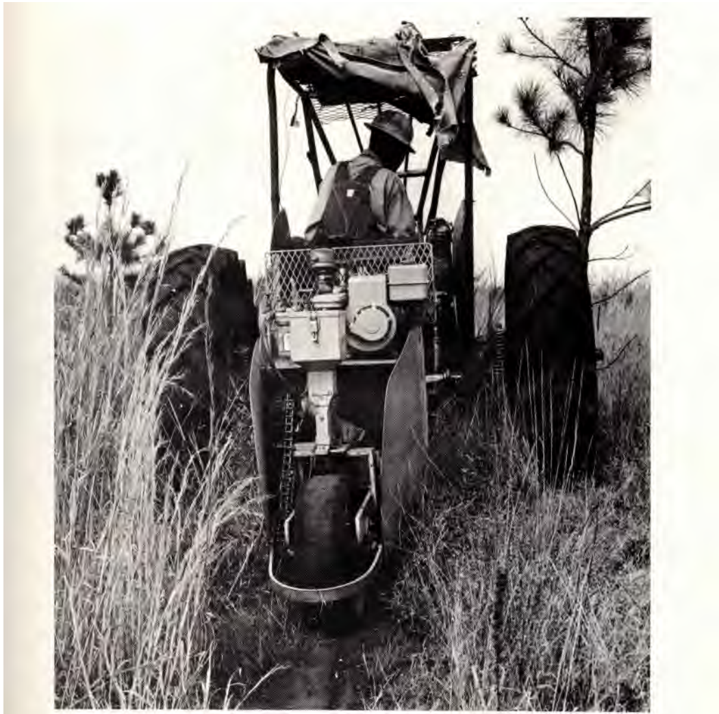
Figure 1.--The new pine seeder, a pneumatically operated seeding system, mounted on a standard furrow seeder, gave good results in pine planting tests. The machine is seeding longleaf pine at the Tuskegee National Forest.
