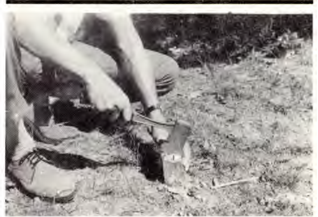
Figure 1.--Cut an "X" in the bottom of each can with a hatchet or other available tool.
