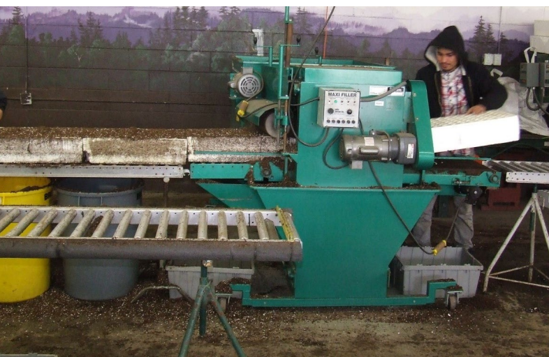
Figure 9. Styroblocks are “loose filled,” where media drops directly into empty cavities. Photo by Nabil Khadduri, USDA Forest Service, 2023.
