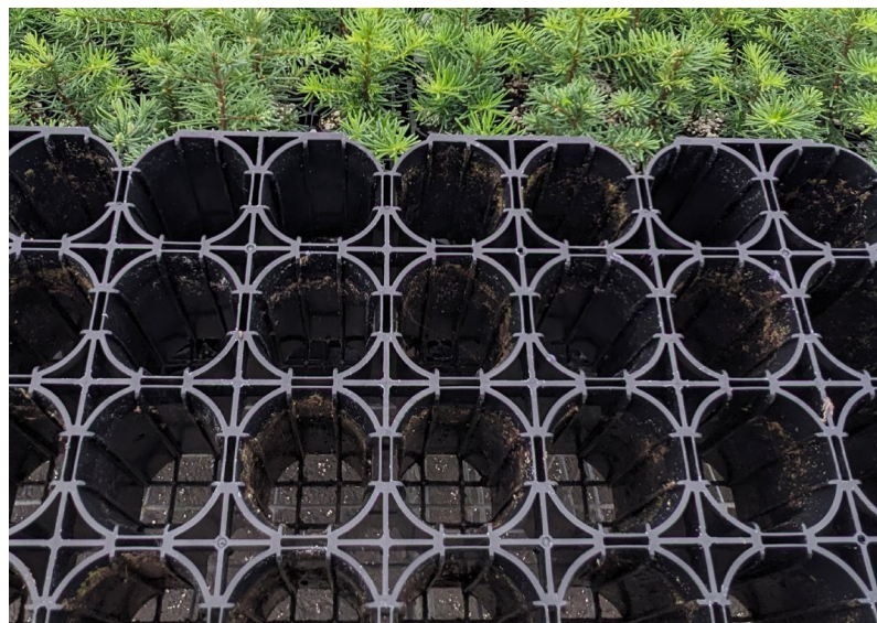
Figure 12. The sturdier injection-molded Proptek 32-count trays (Blackmore Company, Belleville, MI) tested in 2023 had larger ribs and a wide opening at the bottom of the cell that improved air pruning. Photo by Nabil Khadduri, USDA Forest Service, 2023.
