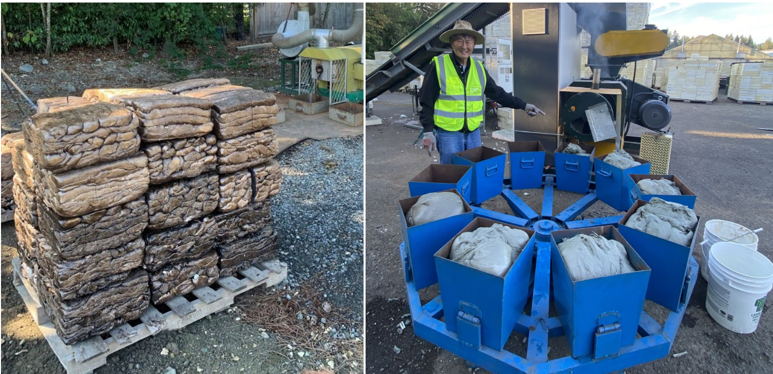
Figure 4. Recently introduced recycling options for Styroblocks include a semi-portable densifier (a) and a service that densifies on site (b). Photo (a) by Steven Kiiskila, Arbutus Grove Nursery, 2023; photo (b) courtesy of Eric Stuewe, Stuewe and Sons, 2024.
