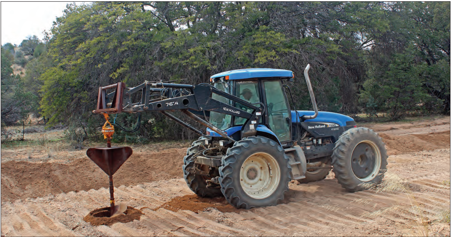
Figure 1. Augers were used to create planting holes that were deep enough for the coyote willow poles. (Photo by Erin Evans, 2012)
