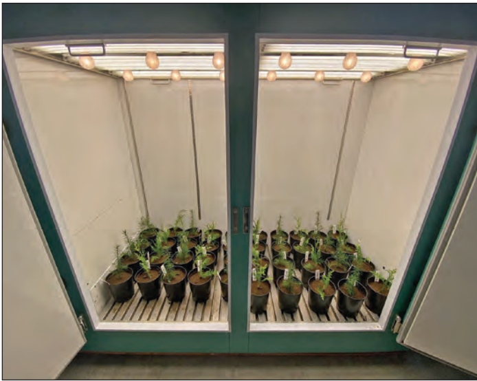
Figure 2. Western redcedar and coastal Douglas-fir seedlings were placed in growth chambers to determine root growth potential following varying cold-storage durations. (Photo by Jennifer Baker, 2022)
