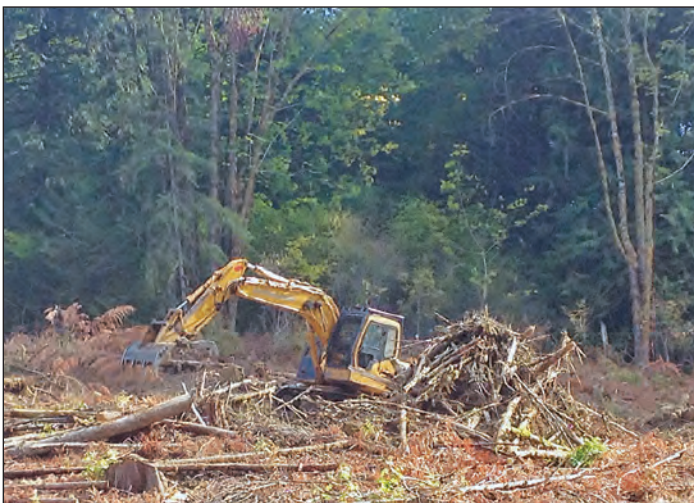
Figure 16. Postharvest piling of slash is a first step in site preparation for planting. (Photo by Glenn Ahrens, 2015)
