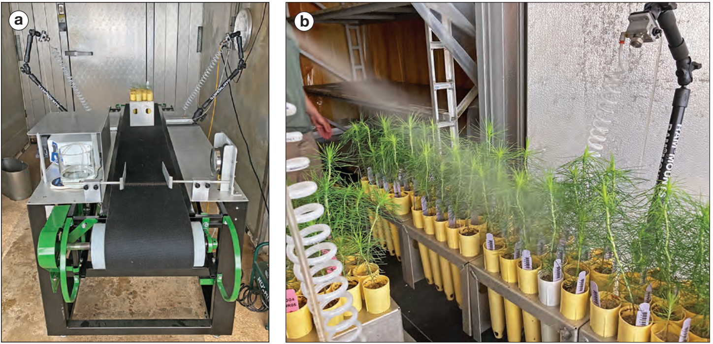
Figure 3. (a) An automated, concentrated basidiospore spray system was developed to mist rust spores onto pine seedling foliage. (b) Specialized nozzles mounted on articulating arms deliver a calibrated volume of aerosolized spore spray as trees move at a constant rate of speed on a conveyer belt. (Photo by Katie McKeever, 2021)
