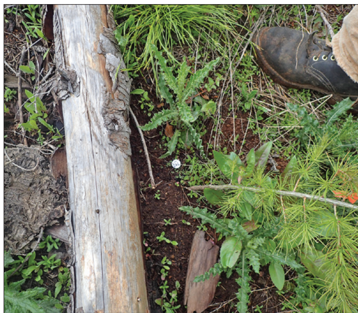
Figure 6. iButton sensors (silver button near the seedling base) were buried immediately below the soil surface near each seedling to measure soil temperature throughout the two growing seasons. (Photo by Andrew Nelson)
