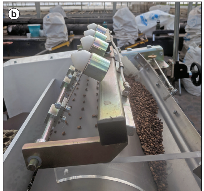
Figure 5. Automated seeders, such as (a) the vacuum needle seeder and (b) the vacuum drum seeder, speed up sowing and increase sowing accuracy. While expensive, increased time savings and seed-use efficiency will quickly recoup costs. (Photos by Nabil Khadduri, 2022)
