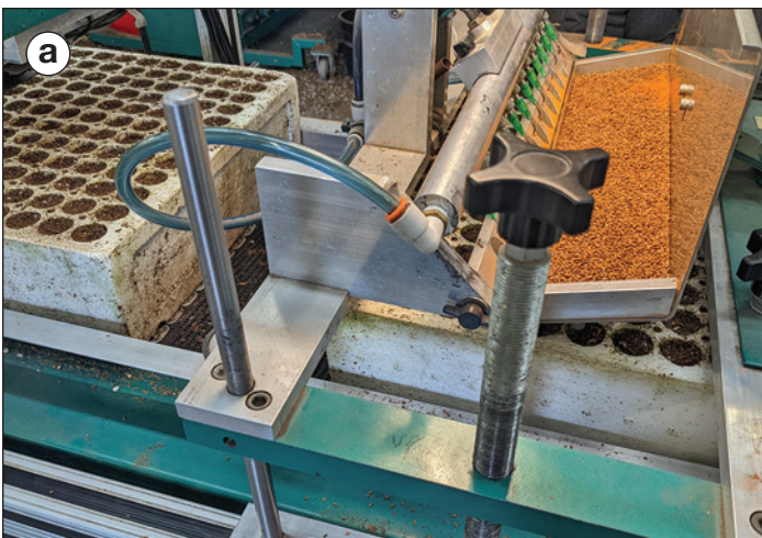
Figure 5. Automated seeders, such as (a) the vacuum needle seeder and (b) the vacuum drum seeder, speed up sowing and increase sowing accuracy. While expensive, increased time savings and seed-use efficiency will quickly recoup costs. (Photos by Nabil Khadduri, 2022)
