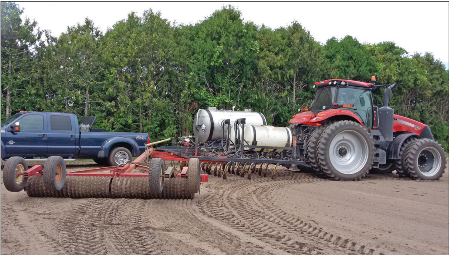
Figure 2. Metam sodium application rig. (Photo by Kyoko Scanlon 2016, Wisconsin Department of Natural Resources)
