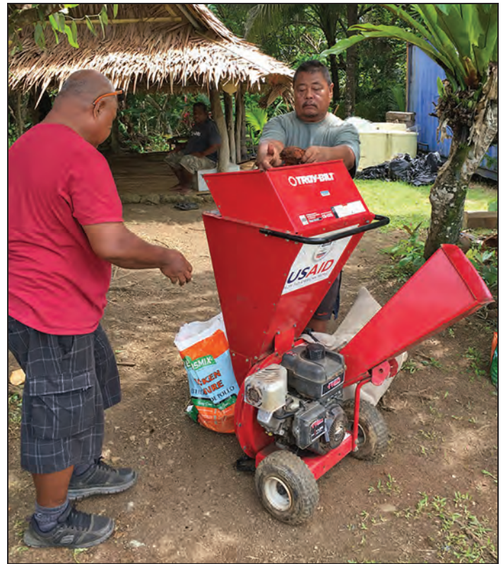
Figure 8. Coconut husks can be shredded using a commercially available chipper-shredder. (Photo by Diane L. Haase)
