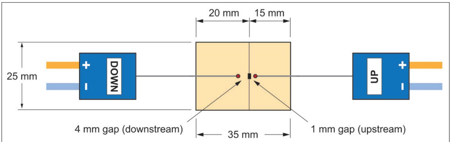
**Figure 2.** Schematic of the sap-flow sensor design. The foam block is represented by the square in the middle. The thermocouples are represented by the small circles and are spaced at 4 mm and 1 mm away from the small resistor chip (small black rectangle).
