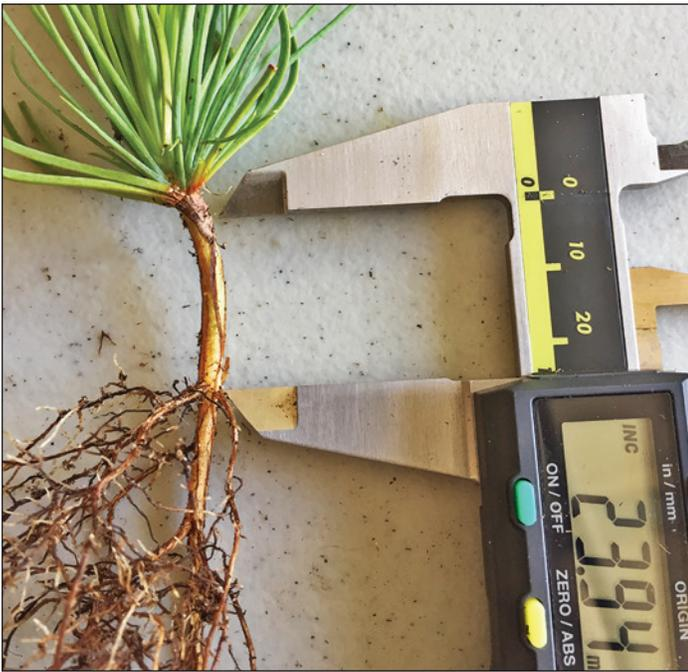
**Figure 6.** A measurement of the entire hypocotyl on a seedling from the base of the cotyledons to the first lateral root (Photo by Paul Jackson 2018)
