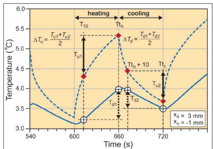
**Figure 4.** With the heat pulse method, temperatures, upstream ( $X_u$ ) and downstream ( $X_d$ ) of the heating resistor are measured by thermocouples. The ( $\Delta T_h$ ) values are measured at 10, 90, 100, and 180 seconds after the start of heating supply. The heat pulse is evidenced by the wave form thermal signature.
