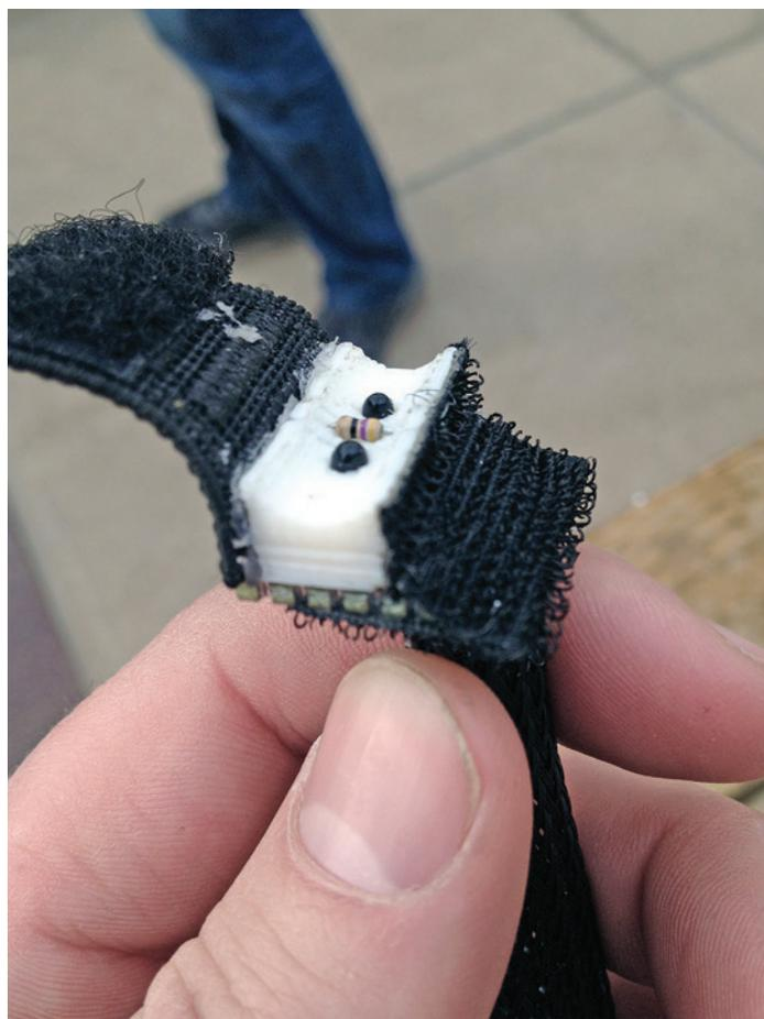
**Figure 1.** Using basic supplies, growers and researchers can construct sap-flow sensors for small-diameter plants. This model is not described in detail but shows how growers can modify the design. For this sensor, we added Velcro® to attach to the stem, used thermistors instead of thermocouples, and used a pile resistor in place of the chip resistor. (Photo by Lloyd Nackley)
