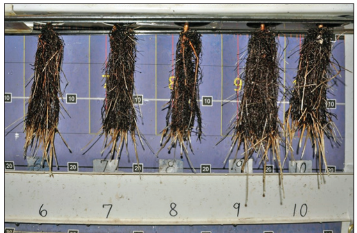
Figure 3. Douglas-fir seedlings after 20 days in a root growth potential test at Center for Forest Nursery and Seedling Research, Seedling Quality Lab at the University of Idaho, spring 2018. (Photo courtesy of Center for Forest Nursery and Seedling Research, Seedling Quality Lab at the University of Idaho, 2018)
