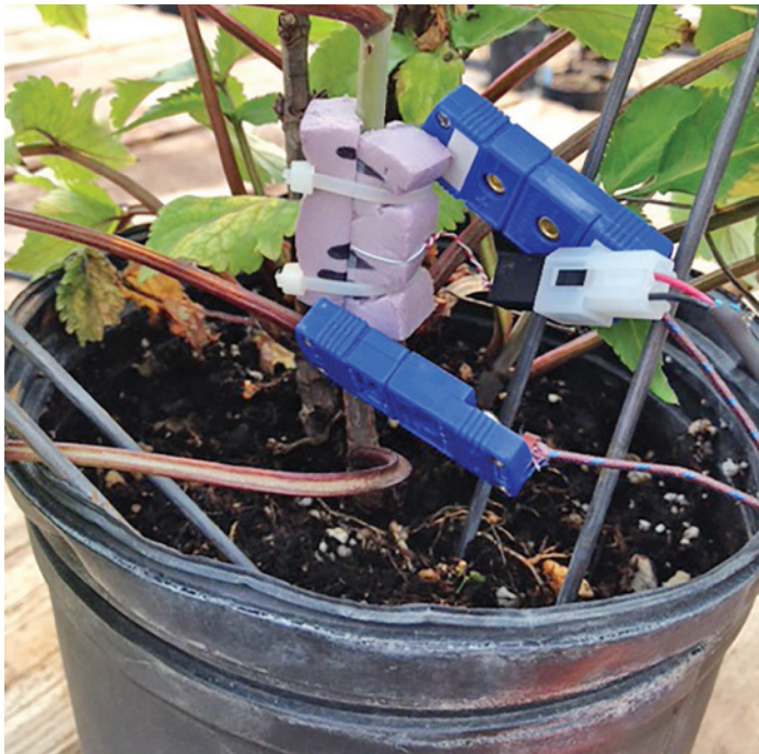
Figure 3. Sap-flow sensor constructed using foam insulation rather than a cork. The sensor is attached to an elderberry seedling ( Sambucus nigra L.). The measurable sap flow is relative to the leaf area downstream (i.e., above) the sensor. Therefore, sensors should be located low on the seedling, or near to the main stem if placed on a lateral branch. (Photo by Lloyd Nackley)
