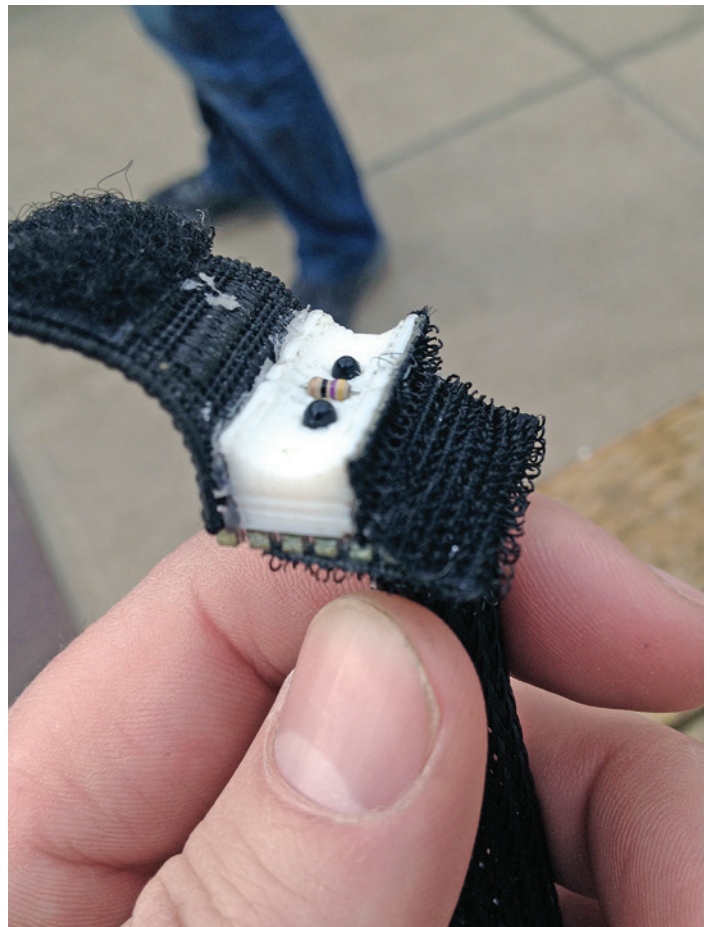
Figure 1. Using basic supplies, growers and researchers can construct sap-flow sensors for small-diameter plants. This model is not described in detail but shows how growers can modify the design. For this sensor, we added Velcro® to attach to the stem, used thermistors instead of thermocouples, and used a pile resistor in place of the chip resistor. (Photo by Lloyd Nackley)
