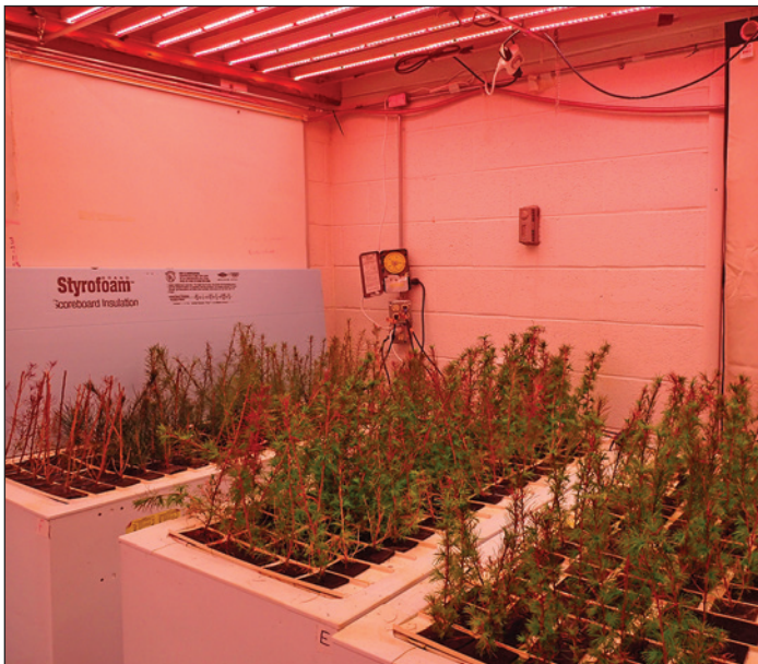
Figure 1. Root growth potential chambers with seedlings suspended on top of the chambers in plastic slats and supplemental light-emitting diode (LED) light bars. (Photo by Andrew Nelson, 2018)
