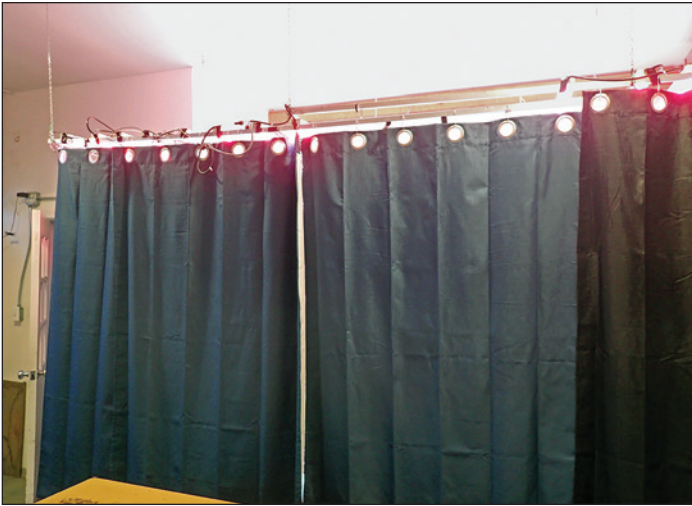
Figure 3. Blackout curtains are suspended from the ceiling around all the chambers. (Photo by Andrew Nelson, 2018)
