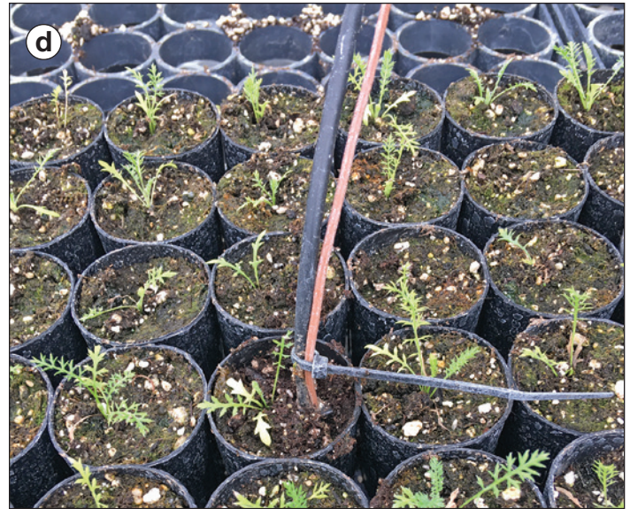
Figure 2. (a) The EC-5 sensor and the Type-T thermocouple used to collect data from small containers in racks. First, (b) an opening was made in the container medium for (c) sensor insertion. After insertion, (d) the medium was filled in around the sensors. (Photos by Steven Link, 2017)
