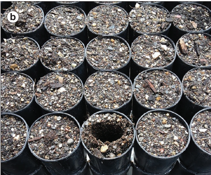
Figure 2. (a) The EC-5 sensor and the Type-T thermocouple used to collect data from small containers in racks. First, (b) an opening was made in the container medium for (c) sensor insertion. After insertion, (d) the medium was filled in around the sensors. (Photos by Steven Link, 2017)
