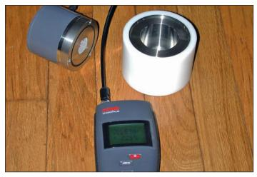
**Figure 3.** Rotronic water activity meter used to measure seed equilibrium relative humidity on small seed samples. (Photo by R.P. Karrfalt 2017)
