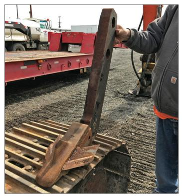
**Figure 5.** This triple-winged shank was used behind a bulldozer for subsoiling treatments on the West Hopper's site. (Photo by Jack Riggin, 2017)
