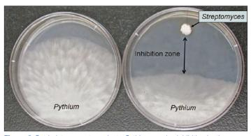
**Figure 8.** Petri plate assay to evaluate *Pythium* species inhibition by the biocontrol agent *Streptomyces lydicus*. No inhibition was observed in plates only containing a *Pythium* isolate (left). Plates containing *S. lydicus* inhibited the growth of *Pythium* toward the other side of the plate, creating an inhibition zone (right). (Photo by Jerry Weiland, 2013)
