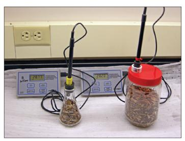
Figure 2. Hygrometers are attached to test chambers to measure seed equilibrium relative humidity. (Photo by R.P. Karrfalt 2017)
