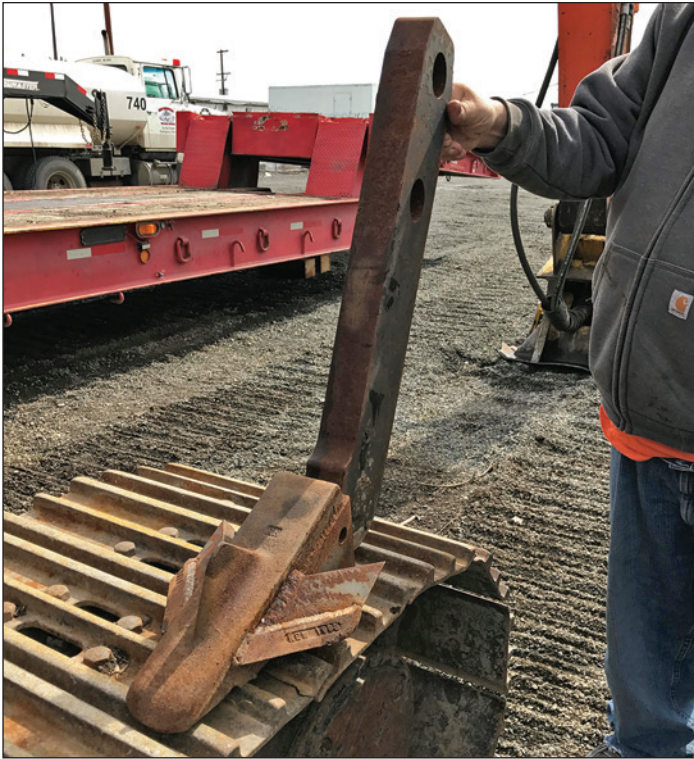
Figure 5. This triple-winged shank was used behind a bulldozer for subsoiling treatments on the West Hopper's site. (Photo by Jack Riggan, 2017)
