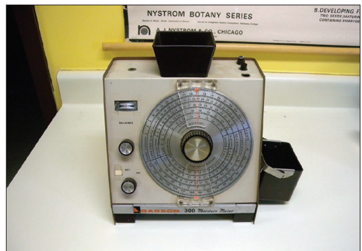
Figure 7. Seed moisture meter that has been used to estimate seed moisture content. (Photo by R.P. Karrfalt 2016)
