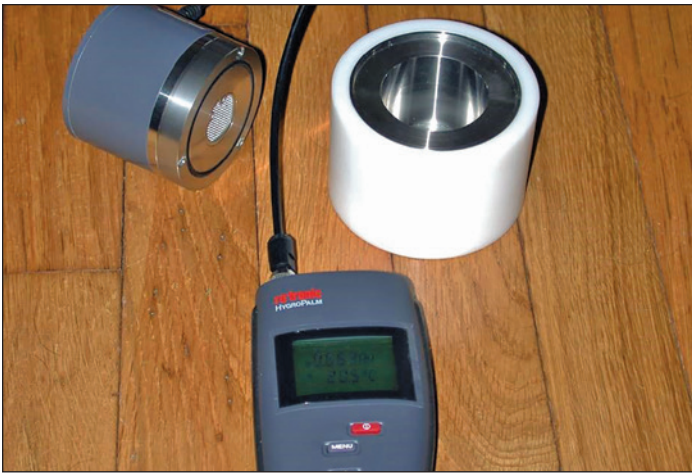
Figure 3. Rotronic water activity meter used to measure seed equilibrium relative humidity on small seed samples. (Photo by R.P. Karrfalt 2017)
