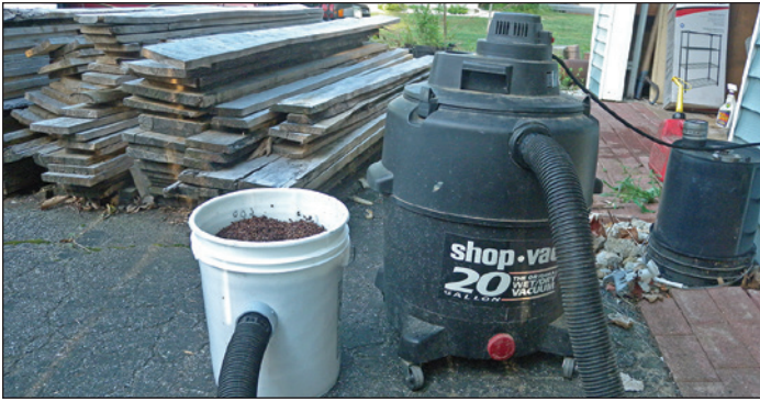
Figure 6. A wet-dry vacuum is used to pull capillary water from the seeds. (Photo by Robert Karrfalt)
