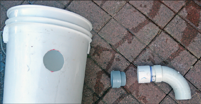
Figure 7. The disassembled base used to hold the paint strainer of seeds during the vacuuming of capillary water. The elbow should point to the bottom of the bucket. (Photo by Robert Karrfalt)
