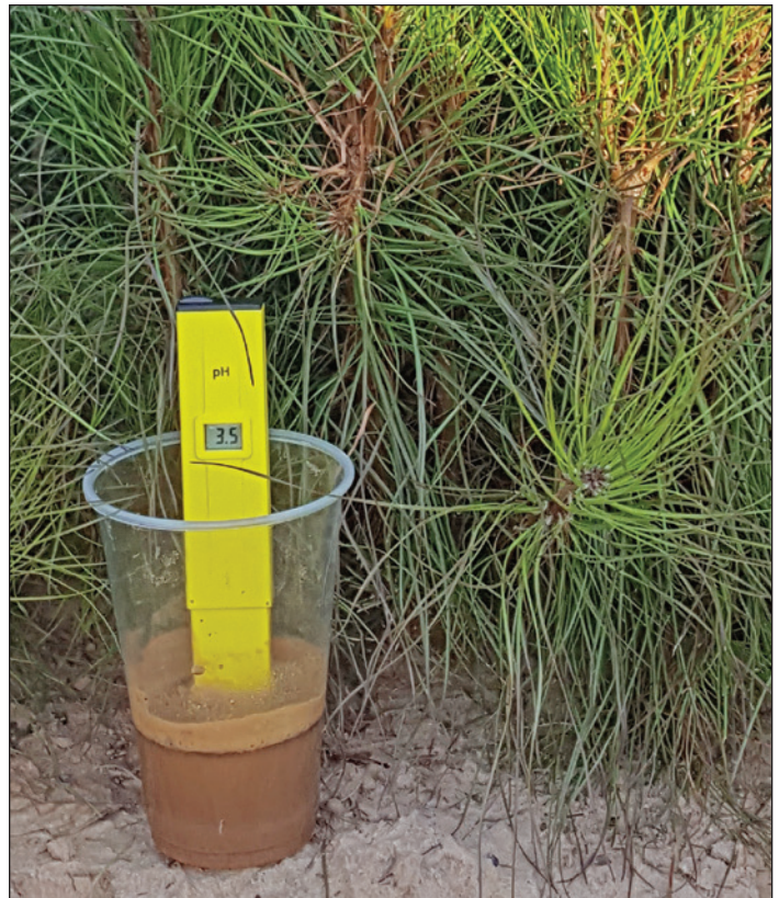
Figure 7. This photo shows loblolly pine ( Pinus taeda ) seedlings (average 32 cm height and 8.2 mm root-collar diameter; measured in February) in pH 3.5 to 3.6 soil. Soil in this plot was treated with 2,440 kg/ha of elemental sulfur on April 9, and seed were sown on April 16, 2016. Rainfall during the 2 weeks following sowing was above average (330 mm total). The topsoil in this plot contained 96 ppm of sulfur in July. If rainfall had been low, however, gypsum crystals (figure 8) might have formed and stunted the seedlings. (Photo by Gene Bickerstaff, Arborgen, 2017).
