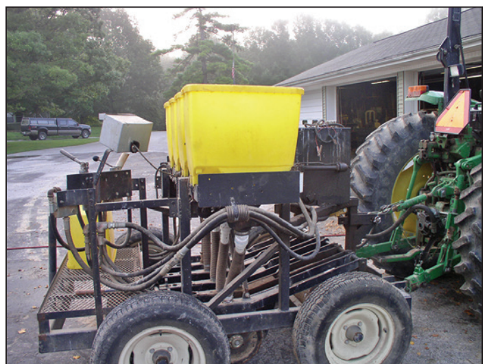
Figure 1. Seeder developed at Indiana's Vallonia State Tree Nursery to achieve target sowing rates for small-seeded acorns and other species with similar-sized seeds. (Photos by Bob Hawkins, 2016)
