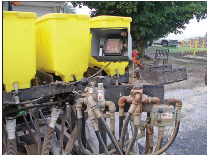
Figure 8. Speed-O-Meter used to control the speed of the seed pickup. (Photo by Bob Hawkins, 2016))
