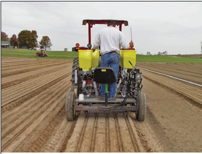
Figure 6. An operator riding on the seeder can monitor and adjust speed and density. (Photo by Jeannie Redicker, 2012)
