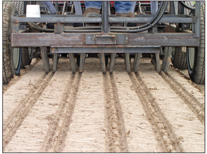
Figure 7. Press wheels used to secure seed into seedbed while covering seed with soil. (Photo by Jeannie Redicker, 2012))
