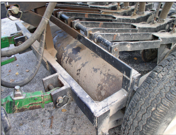
Figure 2. Roller mounted on front of seeder to assist with leveling the seedbed. (Photo by Bob Hawkins, 2016)
