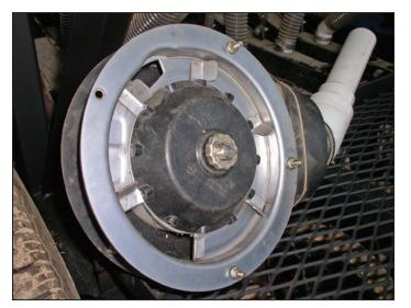
**Figure 3.** Modified finger pickup units used to grab individual seeds for placement in the seedbed. (Photo by Jeannie Redicker, 2012)
