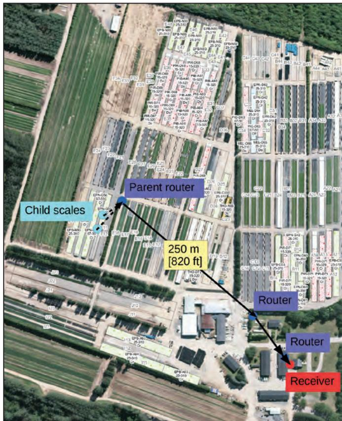
**Figure 5.** Aerial view of Grandes-Piles nursery, Québec, Canada, depicting wireless network scale range obtained in the field. (Extracted from ArcGis by Chantal Pelletier, Grandes-Piles nursery, 2014).
