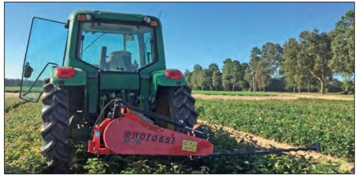
**Figure 1.** Top pruning *Quercus* seedlings using a sickle bar mower at the SuperTree Nursery (Shellman, GA). Only a few, well-replicated top-pruning trials have been conducted in operational hardwood seedbeds. (Photo by Robert Cross, 2008)
