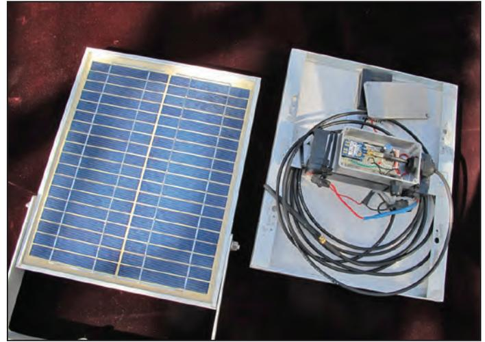
**Figure 3.** A low-cost, stand-alone, solar-powered router (both top and bottom) that uses a 2.3 Ah lead acid 12 V battery charged by a basic 10 W solar shield. The solar shield uses no costly charging regulator, only a diode to avoid battery discharge into the solar shield during the night. With the constant battery demand from the radio, the battery will never be overcharged. (Photo by Daniel Girard, 2016)
