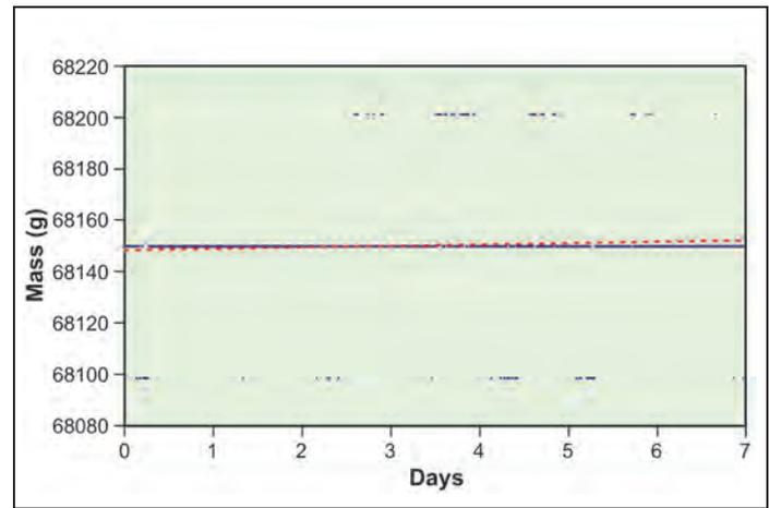
**Figure 10.** The mass overestimation that is generated by creeping represents 0.546 g (0.0182 oz) per day (red dashed line) meaning around 100 g (3.33 oz) for a 200-day growing season. This estimation represents less than 0.3 percent of substrate volumetric water content and is nonsignificant. Thus, the scale has to be calibrated only once a year. (Note that steps between levels of the blue dots represent the resolution of the scale.)
