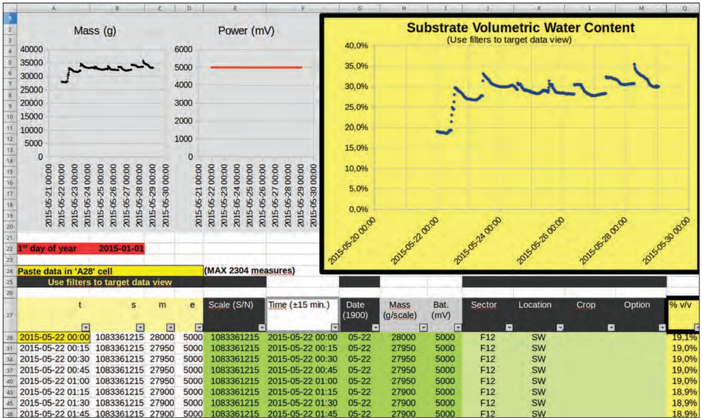
**Figure 12.** An example graph of substrate volumetric water content monitoring (yellow) obtained at Normandin nursery (Québec, Canada). Other graphs (from left to right) represent basic weight (in g) and cell power level (in mV), respectively. All graphs are based on the individual values shown in the table.
