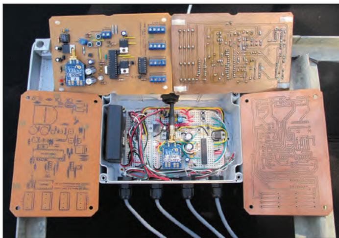
**Figure 8.** The stand-alone scale uses a homemade printed circuit board (PCB) based on Arduino (Ivrea, Italy). First, a draft circuit (in the grey box) was made and tested under field conditions using a solderless board. Thereafter, a homemade PCB was designed and assembled (around the grey box: different production phases). (Photo by Daniel Girard, 2016)
