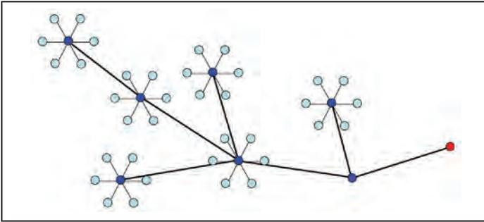
**Figure 1.** Example sketch of a wireless network (cluster tree type). Stand-alone scales (light blue) are powered by cells, and routers (deep blue) are powered using a solar shield. Each router relays the scale data in multiple hops (of no more than 200 m [610 ft] each) to expand the global network range to a single receiver (red) located at the nursery office.
