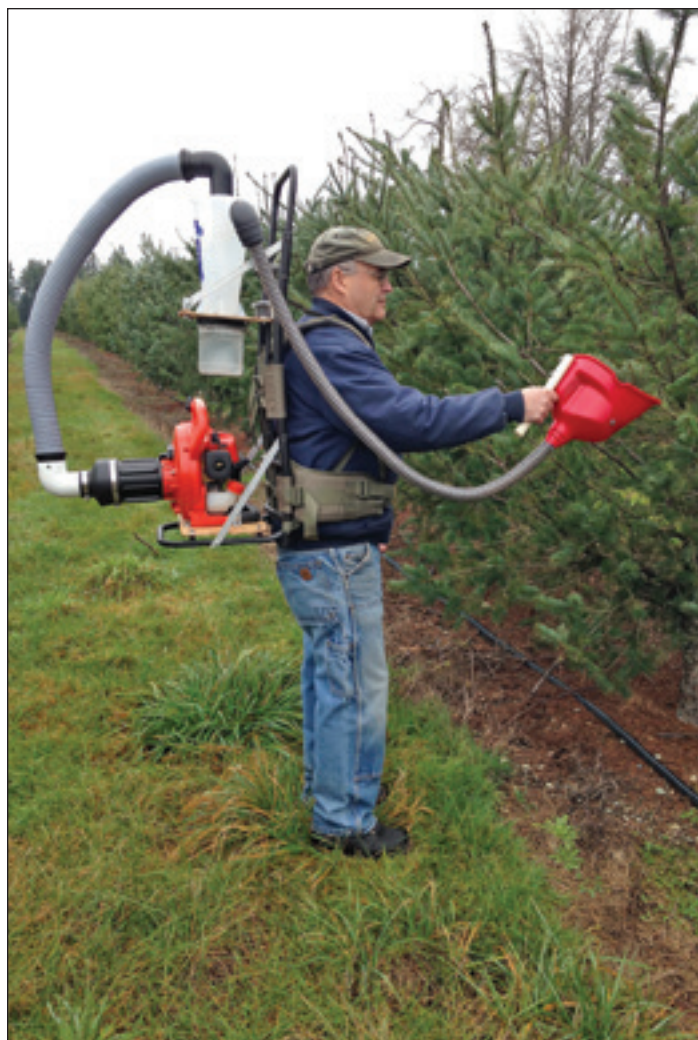
Figure 3. Using the Meridian Pollen Vacuum System, one person can collect more than 0.5 qt (500 cc) of pollen per hour under good shedding conditions. (Photo by Rocky Oster, 2015)
