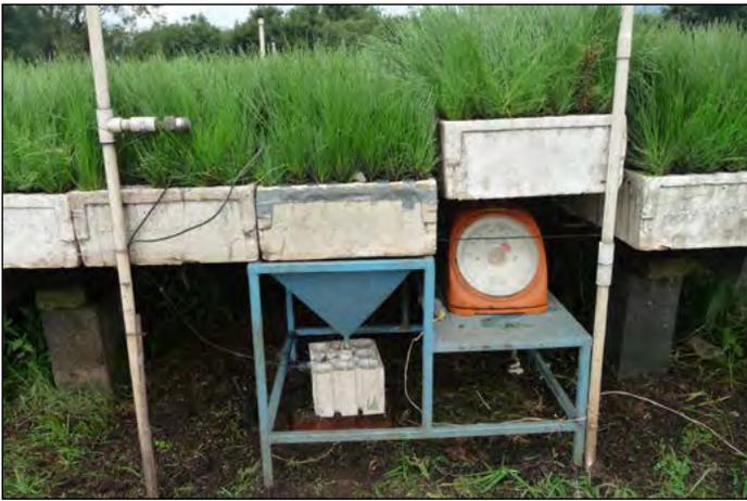
**Figure 1.** Monitoring station in a *Pinus montezumae* Lamb. seedling crop in Copperblock® 60/250ml (15 in<sup>3</sup>; Beaver Plastics Ltd., Alberta, Canada) to measure irrigation, electrical conductivity, block weight, and air temperature. (Photo by Jol Hodgson, 2012)
