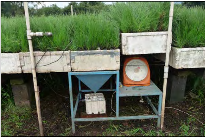
Figure 1. Monitoring station in a Pinus montezumae Lamb. seedling crop in Copperblock® 60/250ml (15 in 3 ; Beaver Plastics Ltd., Alberta, Canada) to measure irrigation, electrical conductivity, block weight, and air temperature. (Photo by Jol Hodgson, 2012)
