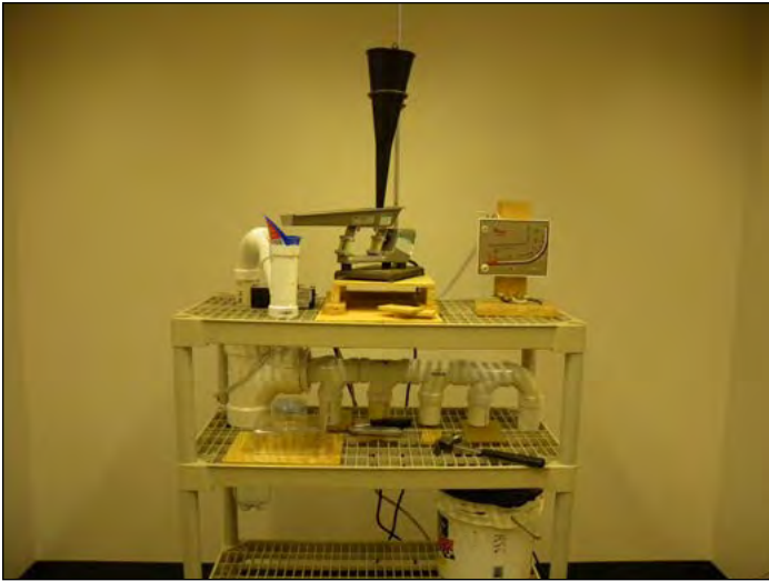
Figure 4. Seed aspirator constructed from PVC (polyvinyl chloride) drainpipe. (Photo by R.P. Karrfalt, 2014)
