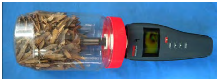
Figure 1. Equilibrium relative humidity of seeds being measured with a hygrometer. (Photo by R.P. Karrfalt, 2012)
