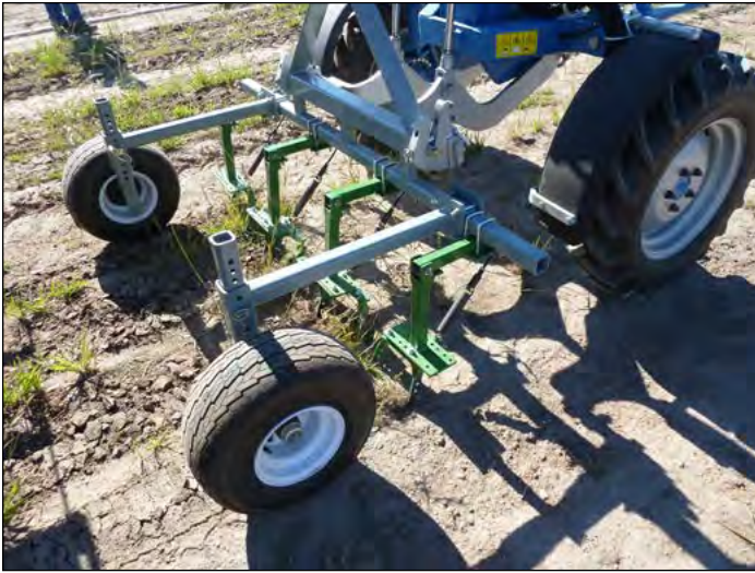
Figure 3. Technology and Development program knife cultivator mounted on the Mazzotti mid-mount tractor. (Photo by Gary Kees, 2012)
