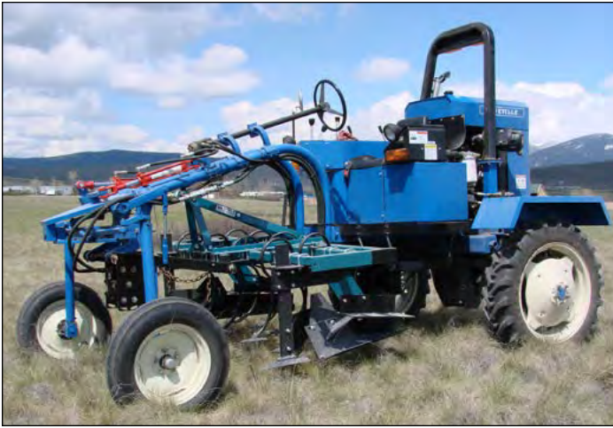
Figure 2. Saukville mid-mount tractor with cultivator. (Photo by Gary Kees, 2010)
