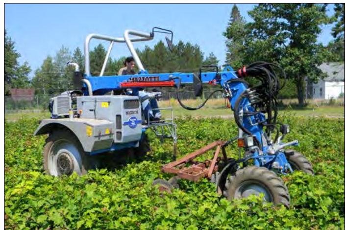
Figure 1. Mazzotti mid-mount tractor cultivating a red oak seedling bed. (Photo by Christy Makuck, USDA Forest Service, 2012)
