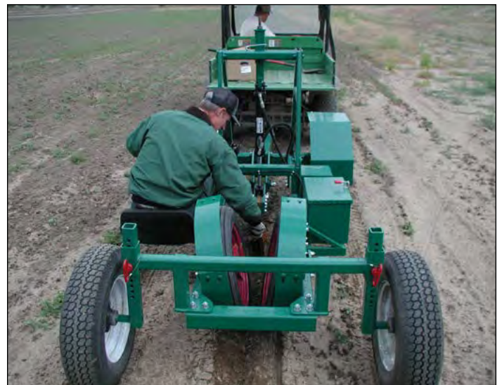
Figure 5. The utility terrain vehicle (UTV) tree planter for planting seedlings at the Lucky Peak Nursery. (Photo by Clark Fleege, USDA Forest Service, 2014)
