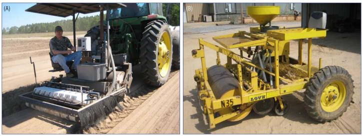
Figure 2. Machines used to sow a bareroot nursery (A) Vacuum precision drum sower (Silver Mountain Equipment<sup>®</sup>) and (B) Gravity drop sower (Love<sup>®</sup>). (Photos by Tom Starkey, 2009 and 2014)
