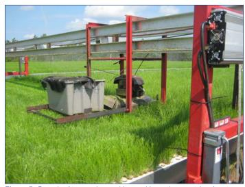
**Figure 5.** Example of top pruning machine used in southern container forest nurseries. These machines are custom designed and manufactured locally to accommodate individual nursery configuration. (Photo by Tom Starkey 2009)
