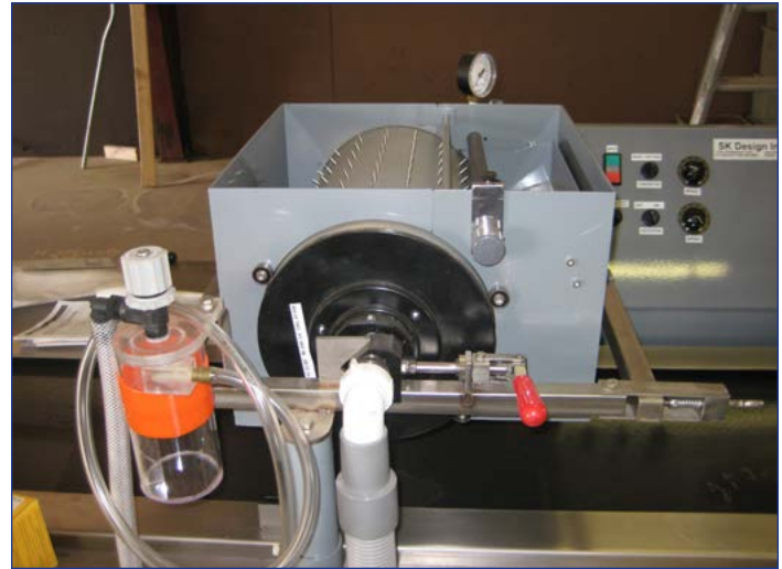
Figure 3. Vacuum-drum sowing machines (SK Design, Inc.) are used by larger container nurseries. These sowers are capable of sowing 300,000 to 400,000 cavities a day. (Photo by Tom Starkey 2009)
