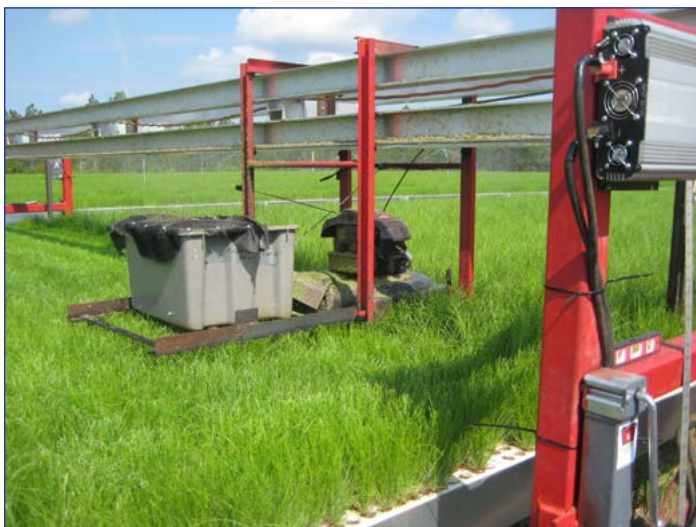
Figure 5. Example of top pruning machine used in southern container forest nurseries. These machines are custom designed and manufactured locally to accommodate individual nursery configuration. (Photo by Tom Starkey 2009)
