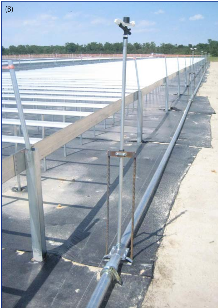
Figure 4. Irrigation systems used in southern container forest nurseries include (A) a center pivot irrigation system on benches and (B) a stationary impact head on a “T”-rail bench system. (Photos by Tom Starkey 2009 and 2010)
