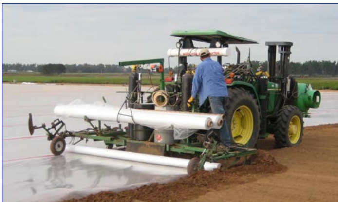
Figure 5. Fumigation of bareroot nursery with methyl bromide/chloropicrin under plastic. (Photo by Tom Starkey 2008)
