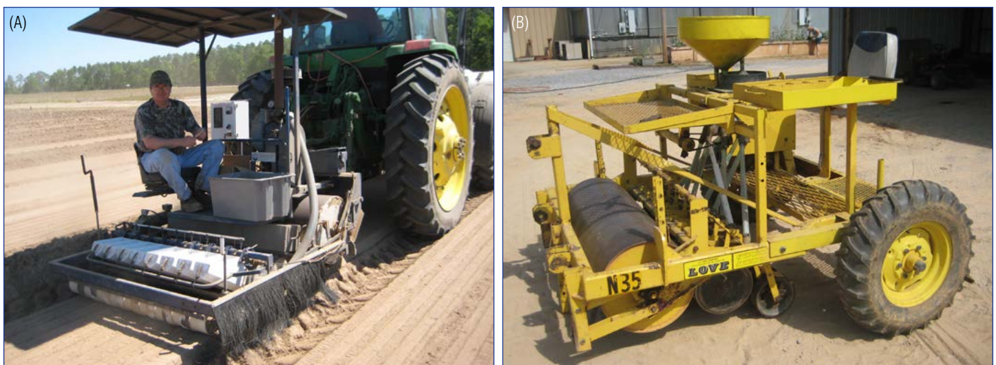
Figure 2. Machines used to sow a bareroot nursery (A) Vacuum precision drum sower (Silver Mountain Equipment®) and (B) Gravity drop sower (Love®). (Photos by Tom Starkey, 2009 and 2014)
