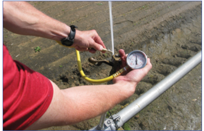
Figure 5. Measuring water pressure with a pressure gauge attached to a pitot tube. (Photo by Ronald Overton 2013)
