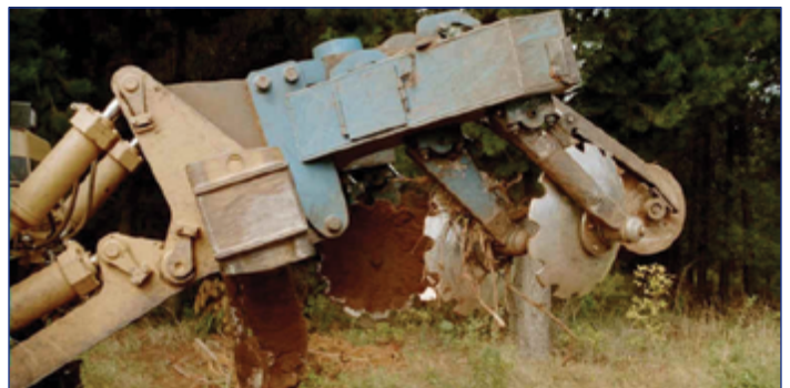
Figure 1. Typical 3-in-1 combination plow used for tillage showing disks for surface tillage and ripping shank for subsoil tillage. (Photo by Forest Productivity Cooperative, North Carolina State University, date unknown)
