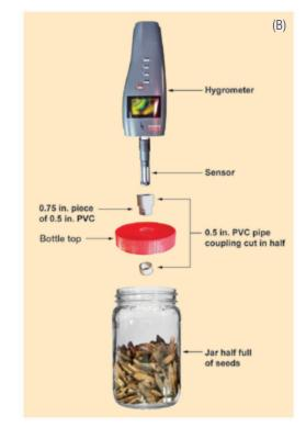
**Figure 3.** (A) Hygrometer inserted into closed jar to measure the equilibrium relative humidity of a seed sample. (B) Schematic representation of the hygrometer, insertion port, and sample jar. (Photo by Robert Karrfat and illustration by Jim Marin)
