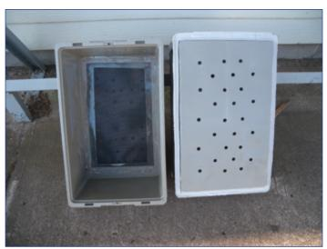
**Figure 10.** Box on the left shows pet screen taped to the bottom and box on the right shows hole pattern and foam gasket. (Photo by Robert Karrfalt)
