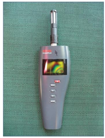
**Figure 2.** Hand-held hygrometer for measuring relative humidity in drying area and equilibrium relative humidity of seed samples. (Photo by Robert Karrfalt)
