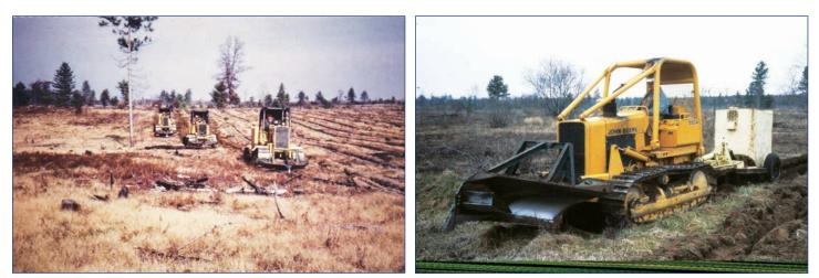
Figure 5. Whitfield planting machines (left and right) mounted on John Deere bulldozers were used for several years, circa 1980. (Photos from MDNR files)
