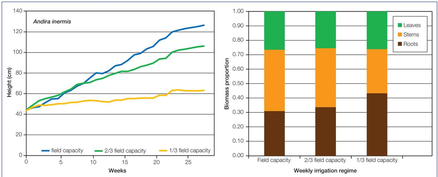
Figure 7. Height growth (left) and biomass proportioning (right) of *Andira inermis* trees subjected to three irrigation regimes.
