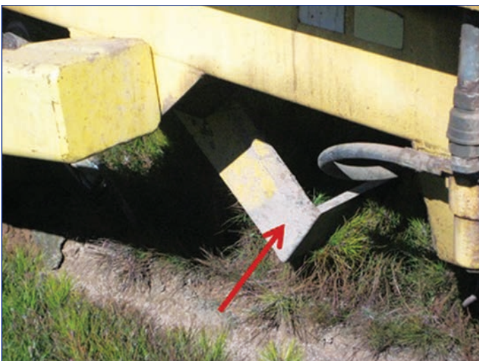
Figure 8. Love® full-bed lifter with seedling lifter bar in raised (unused) position (top) and in lowered (in use) position (bottom). (Photo by Tom E. Starkey [top] and Ben Whitaker, Auburn University [bottom])
