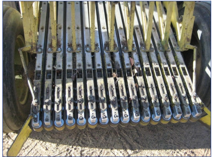
Figure 5. Lifter belts for the Love® full-bed seedling lifter. Each of the two adjacent belts lifts one row of seedlings. (Photo by Tom E. Starkey)
