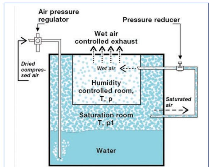
**Figure 2.** Schematic diagram of a two-pressure reactor.  $T$  = temperature,  $p_1$  = saturation pressure, and  $p$  = post-expansion air pressure. (Adapted from HUMOR 20 High-precision Humidity Calibrator data sheet, E + E Elektronik Ges.m.b.H, Langwiesen 7, A-4209, Engerwitzdorf, Austria)
