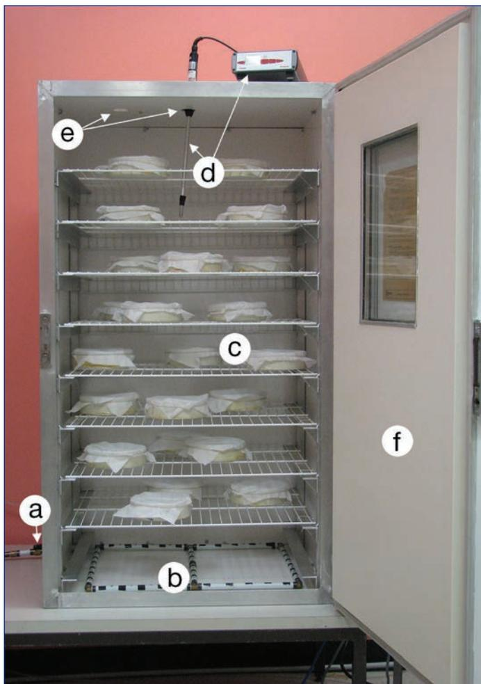
**Figure 6.** Drying cabinet built at the Direction de la recherche forestière. (a) Drying air intake at controlled humidity levels, (b) air intake suitable for the final expansion of drying air, (c) containers used for drying pollen lots, (d) hygrometry probe in the drying cabinet, (e) outlets to evacuate drying air after use, (f) drying cabinet door. (Photo by Fabienne Colas, 2012)
