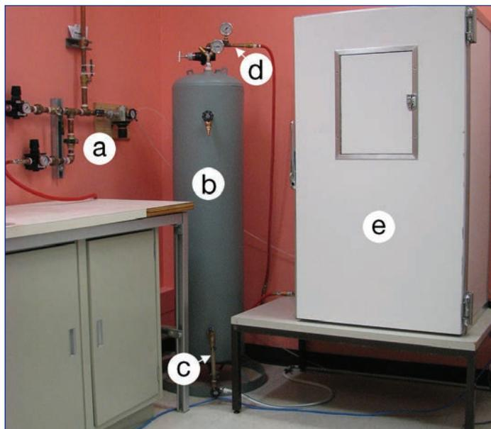
**Figure 4.** A general view of the device installed at the laboratory of the Direction de la recherche forestière. (a) Compressed air supply (in this case, supplied by the building system); (b) saturation tank (air humidification); (c) control tube showing the level of water in the saturation tank; (d) outlet for driving air at a predetermined level of  $a_w$  into the drying cabinet; (e) drying cabinet. (Photo by Fabienne Colas, 2012)
