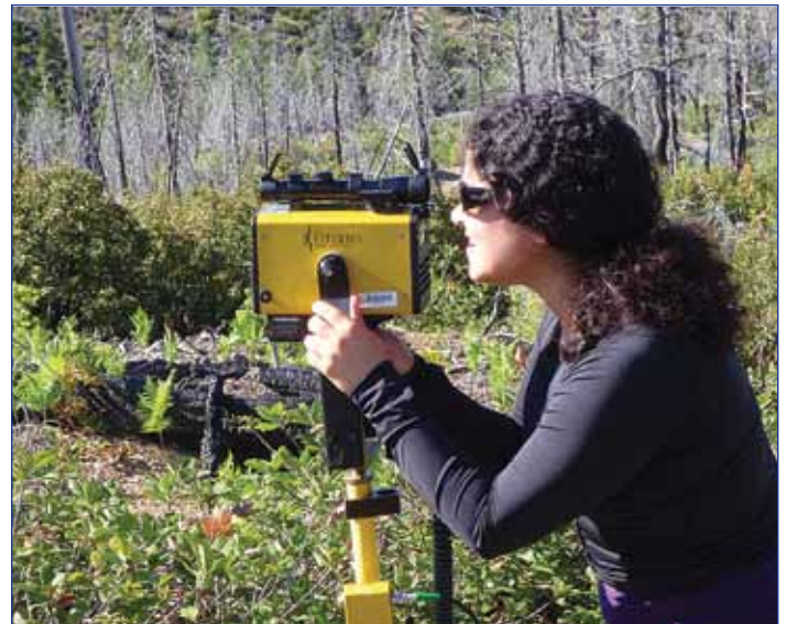
Figure 2. The position and characteristics of each woody plant in every plot was surveyed using a reflector paddle (left) and Criterion Electronic Laser surveying instrument (right). (Photo source: Diane L. Haase 2008).
