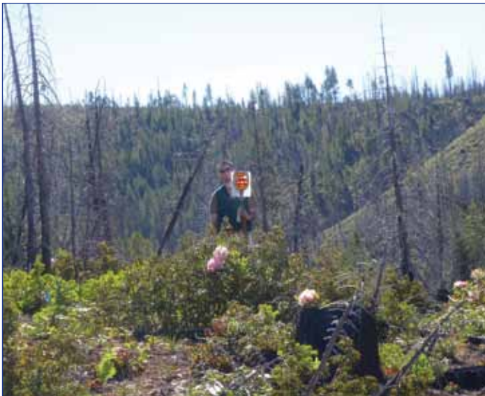
Figure 2. The position and characteristics of each woody plant in every plot was surveyed using a reflector paddle (left) and Criterion Electronic Laser surveying instrument (right). (Photo source: Diane L. Haase 2008).
