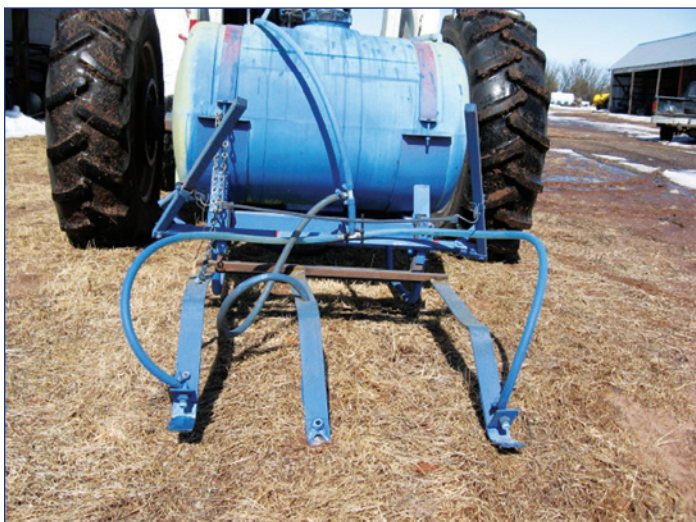
Figure 4. Nozzle placement on sprayer (Photo source: Theresa Dobosenski, Minnesota Department of Natural Resources, 2011).
