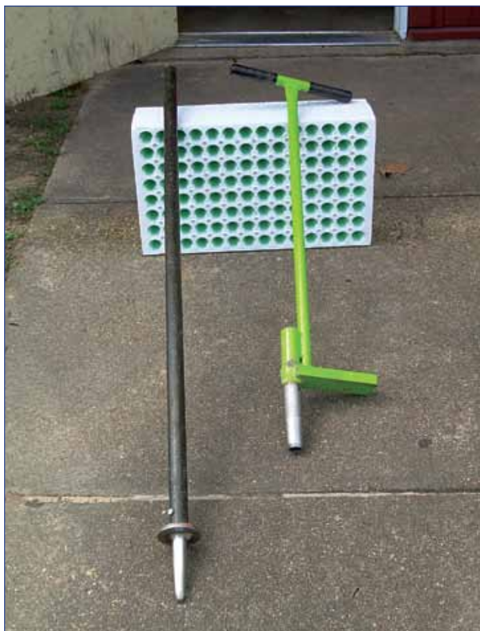
Figure 1. The tool on the left is the solid round dibble with a bit made in the shape of a container cavity, such as those used for growing the seedlings in this study. The tool on the right is a tube dibble that is available commercially from several sources. Both tools are leaning on a Copperblock™ Beaver Plastics Styroblock, model number 112/105, which was the type of container used to grow the longleaf seedlings in this study.
